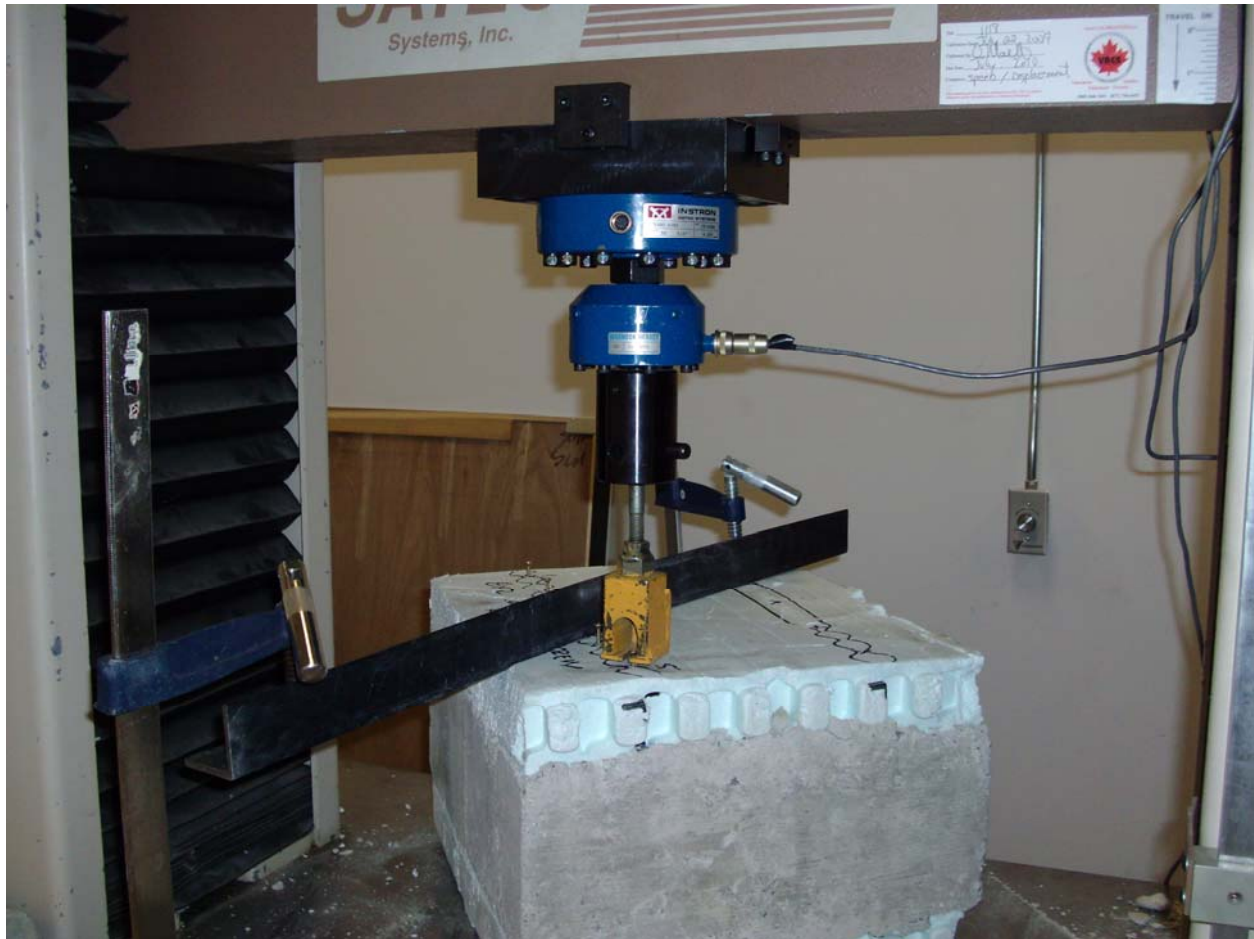
Photograph No. 14: Showing test set-up for screw and nail withdrawal test using Satec Unidrive Testing Machine.
