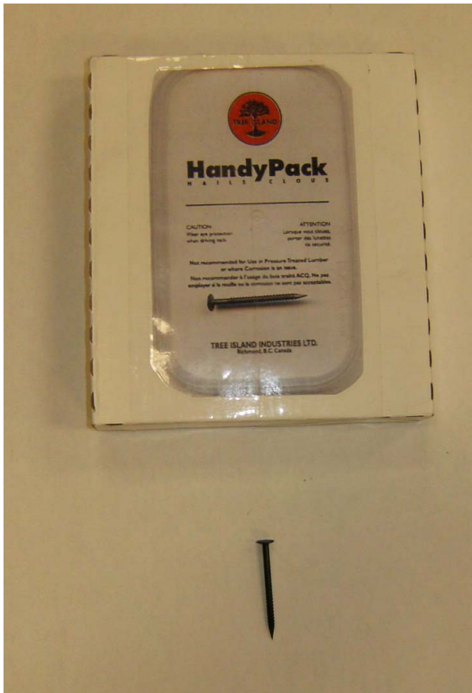
Photograph No. 12: Showing Tree Island Fasteners 1-1/2" Ring Nails
