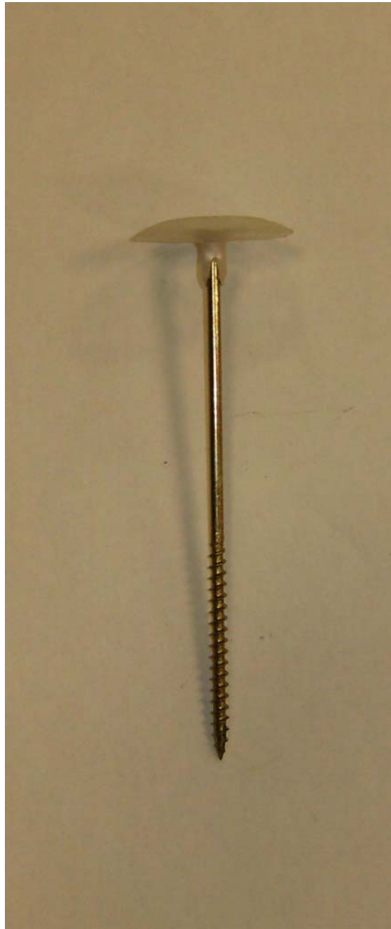
Photograph No. 13: Showing Fastener 6" Brick Ledge Screws
