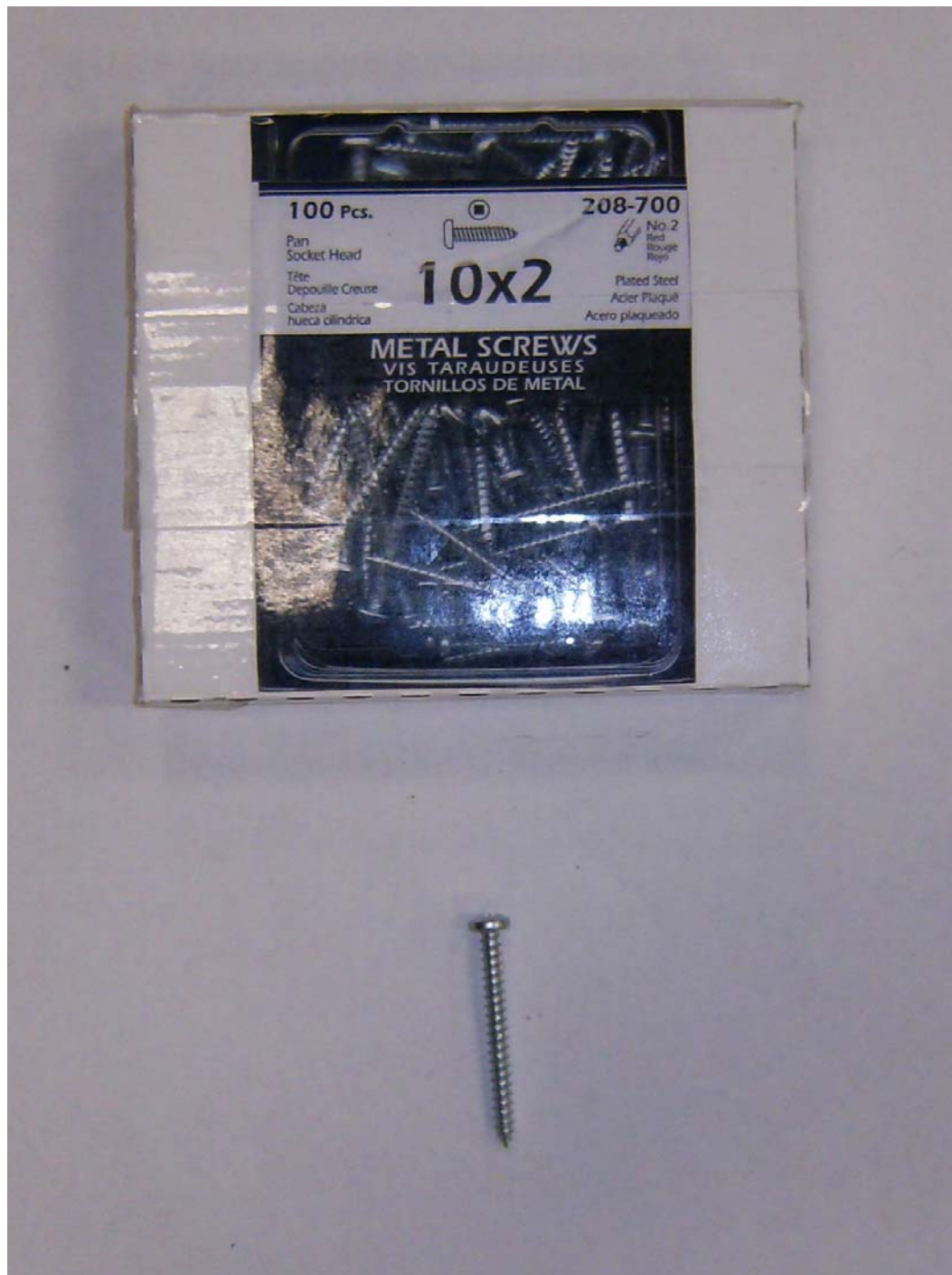
Photograph No. 6: Showing Fasteners 10 x 2 Metal Screws Number 208-700
