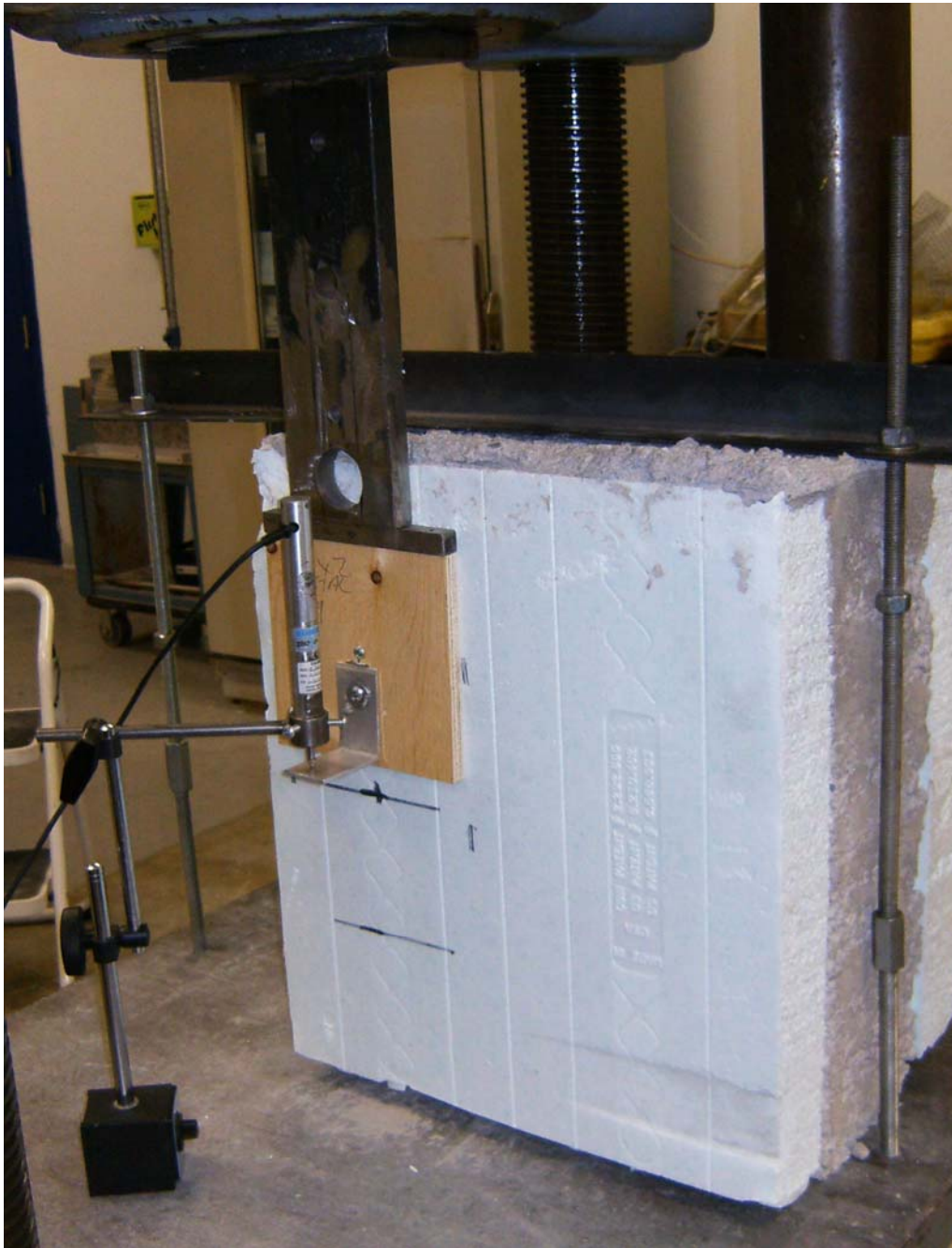
Photograph No. 15: Showing set-up for lateral fastener resistance tests.
