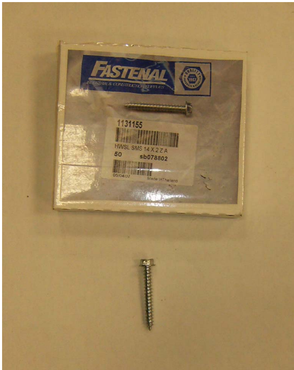
Photograph No. 10: Showing Fasteners Fastenal HWSL SMS 14 X 2 ZA Screws Number 1131155
